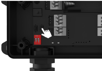
Pairing Button for Slack rope switch
