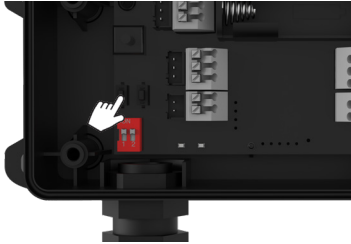
Pairing Button for Safety Edge
